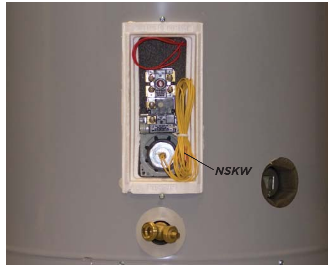
Yellow Thermistor Wires Connected to TB (3 and 4) on NSKW Control Board
