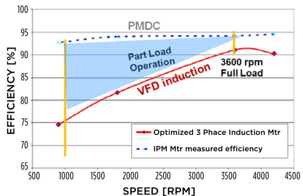
**EC Plenum Fan Efficiency vs a VFD Belt Drive Blower**
