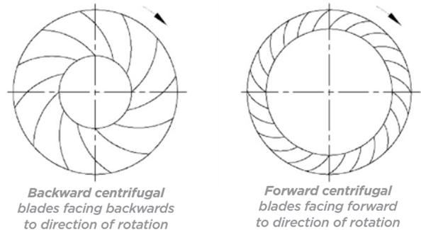
**Forward Curved Fans** operate at lower speeds (typically 900-1400 rpm) and pressures compared to its backward curved counterpart. Backward curved fans (75-80%) have an approximate 10-15% efficiency advantage over the forward curve cousin (65-70%).
