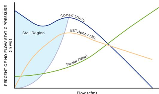
**Backward Curved (Plenum) Fans** operate at higher speeds (typically 900-3000 rpm) and pressures compared to its forward curved counterpart. In the case of integrated EC plenum fans, the fans are factory balanced and provide quiet vibration free operation. Backward curved fans can be used
