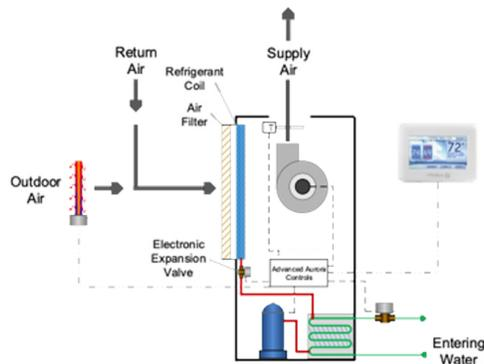
Traditionally, reheating the air leaving the air conditioning system has become the industry standard solution to controlling humidity (Figure 1). The air returning from the conditioned space is cooled well below the dew point in order to condense as much moisture from the air as possible and then it is reheated to a higher temperature, helping to prevent overcooling, before being sent back to
