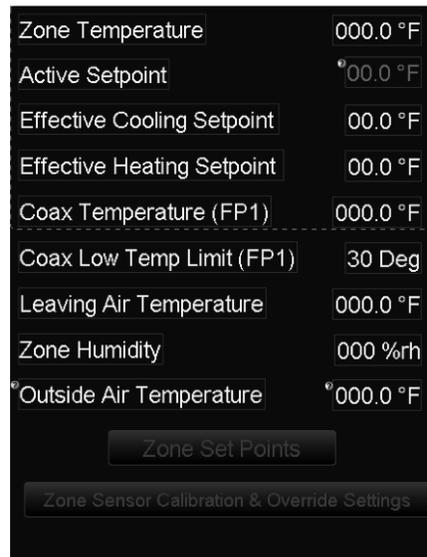
The buttons at the bottom of this page will take you to the associated screen. This provides a quick way to navigate back and forth between the Zone temperature, set points, and calibrations pages. These pages are covered under the “Settings” page of this document.
