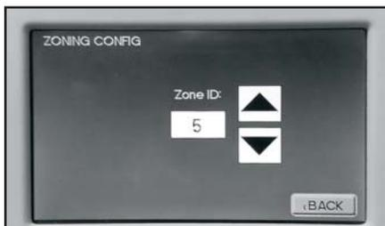
If more than one zone is assigned the same zone number an error will be displayed on the thermostat and MasterStat. After the initial configuration to change the zone numbers enter the configuration mode by holding a finger over the Zone number in the upper left hand corner for 5 sec. Select zone number and use the up/down arrow to adjust.
